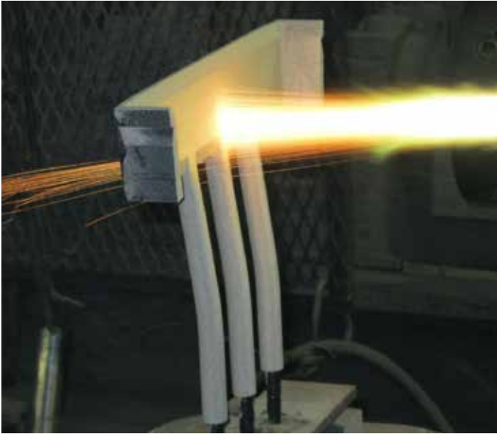
Brick Die Bridge being sprayed with Colmonoy® 62M Powder.
