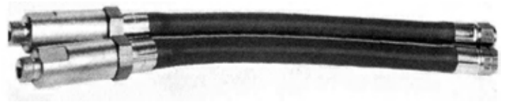
Figure 9-3. Dual flash-back arrestor
