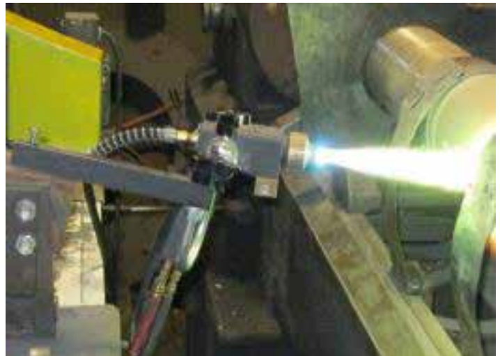
Model J-3 Spraywelder™ mounted on the "Tool Post Holder" spraying Colmonoy® 6 onto a large 8620 shaft. Notice the metal plates used for shadow masking the edges of the spray area.
