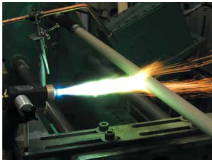
Down hole pump plunger sprayed by a J-3 Spraywelder™. Alloys such as Colmonoy® 5, 5A, 6, 62, 6000 or 6001 can be used for this application depending on the coating hardness desired.
