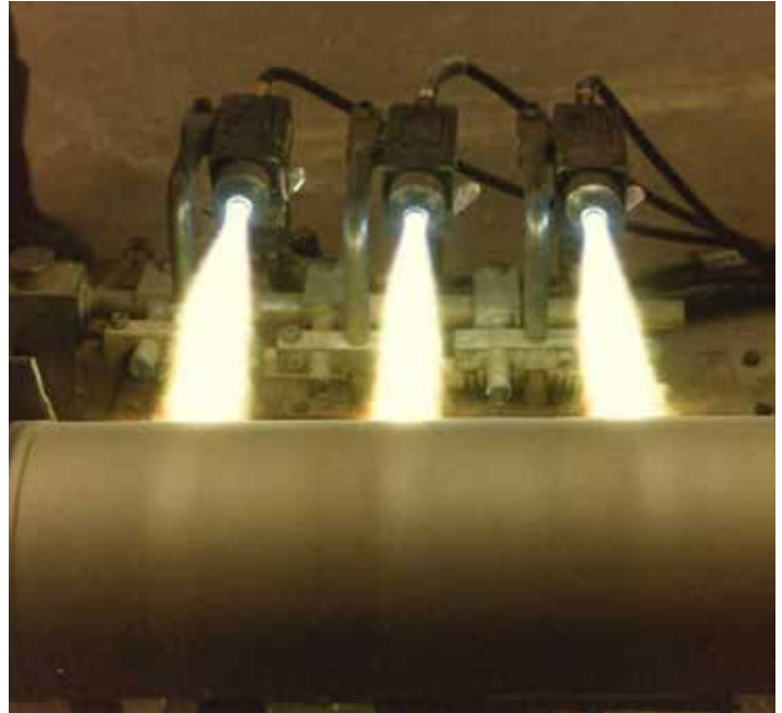
Three model J-3 Spraywelder™ spraying Colmonoy® 5 Powder in tandem on a shaft.
