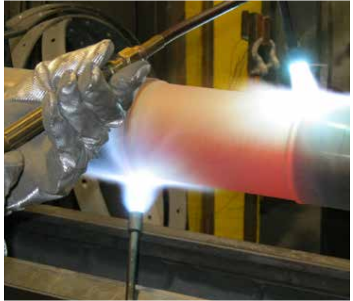
Preparing to fuse Wallex™ 50 on to a large stem of Inconel X-750.
