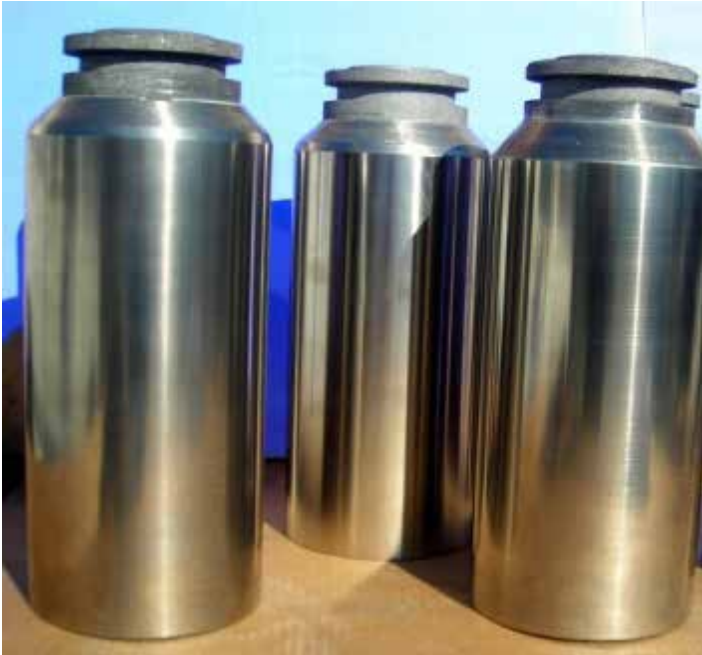
Oil & Gas Frack Pump Plungers Spray and Fused, then ground with Colmonoy® 88 .
