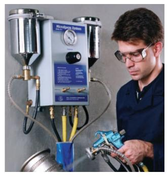
Model N-5 has two powder hoppers. This allows you to operate continuously (switching from one hopper to the other); use both hoppers for higher rates; switch between two different powders; or blend two materials.
