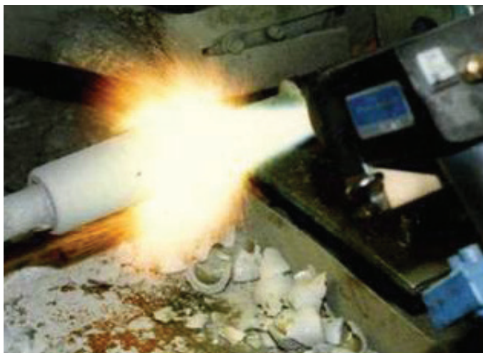
A Sucker Rod Coupling Sprayed and Induction Fused.
