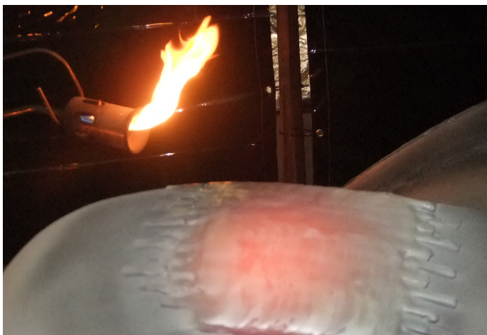
First completed section of as-welded stabiliser by Colmonoy® 25F
