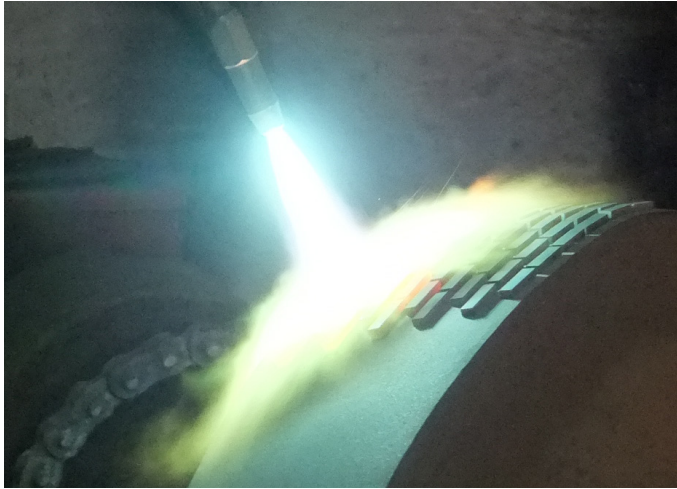
Tungsten carbide inserts being cemented into place using Colmonoy® 25F
