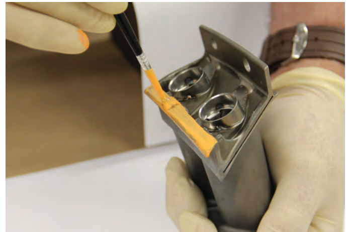
Orange Stop-Off™ brushed on vane segment
