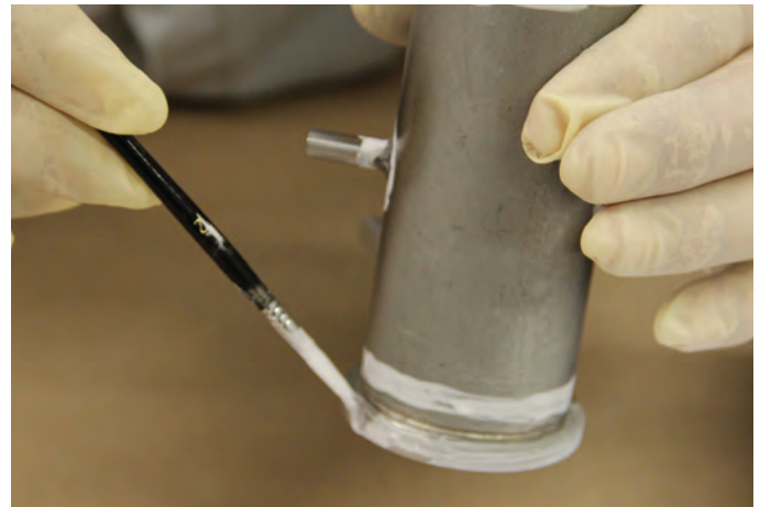
White Stop-Off™ brushed onto bracket
