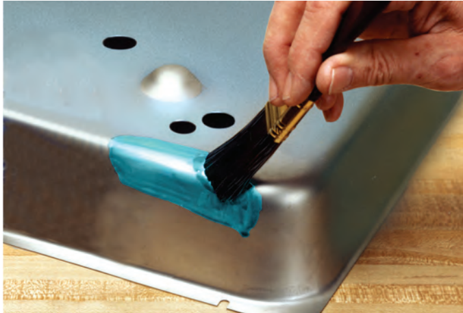
Blue Stop-Off™ brushed onto surface part
