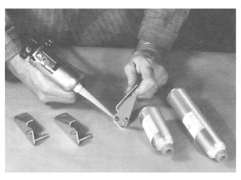
CuBraz Filler metal is powdered copper pre-mixed with a binder. It is easily applied with air-powered applicator, prior to furnace brazing.
