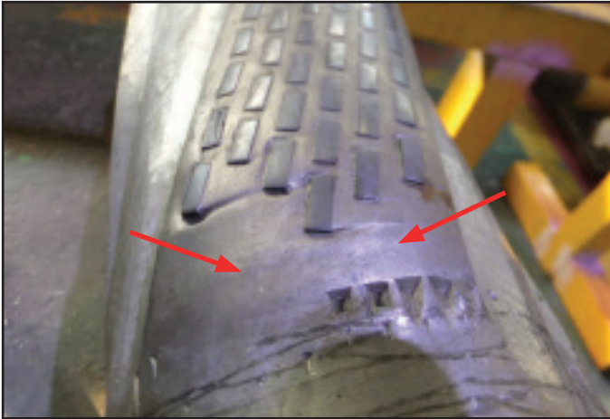
Image shows the leading edge with tile loss and erosion of the cementing matrix powder. Further use would result in rapid tile loss. Colmonoy® 7541-55F improves performance in reducing wear rates in this area
