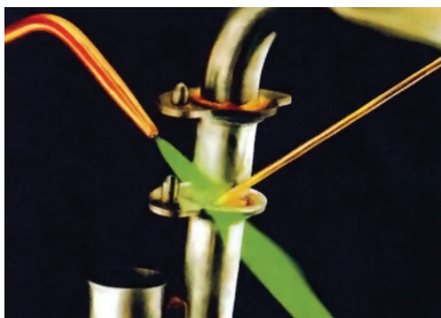
Yellow Stop-Off™ for Torch Brazing image source: AWS Brazing Handbook P. 238
