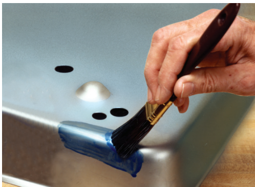
Blue Stop-Off™ brushed onto surface part
