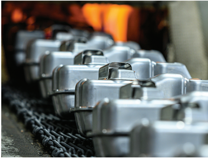
Mufflers used in outdoor equipment to be brazed with Nicrobraz® 5027 in a humpback belt furnace
