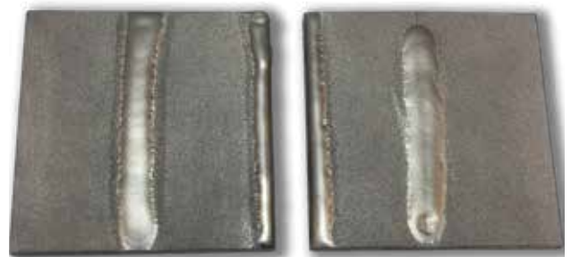
ColWear 62-1 coating gouged to produce significant defects and then repaired using Fusewelder™ Torch & Colmony® 62 powder.
